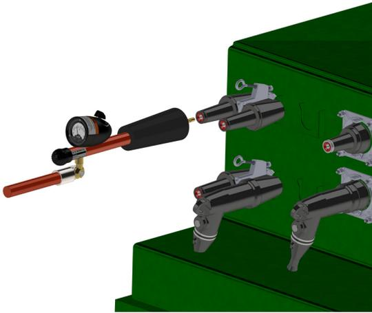
3. Secure a temporary feed-thru device in parking stand on the deadfront transformer or switch. Pull elbow with appropriate hot line tool and install elbow on feed-thru device.
