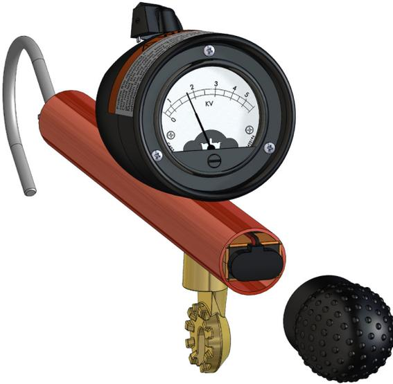
Check meter, battery and circuitry for proper operation before and after each use by depressing test button at back of meter housing while switching selection to each setting in sequence. Set at every position except "Off", meter should read nearly full scale. When reading falls three or four divisions below full scale, replace battery by removing plastic cap on end of mounting stick. Use a 9-volt battery.
